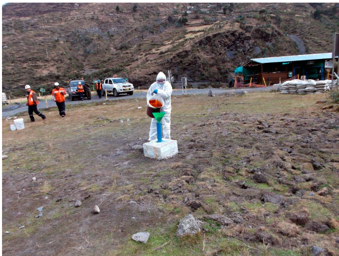
Figure Box 32-1 - Dye introduction into a well. Tyveks are worn to reduce the chance that workers could contaminate a vehicle or other material with dye. Small amounts of dye can penetrate Tyveks.
