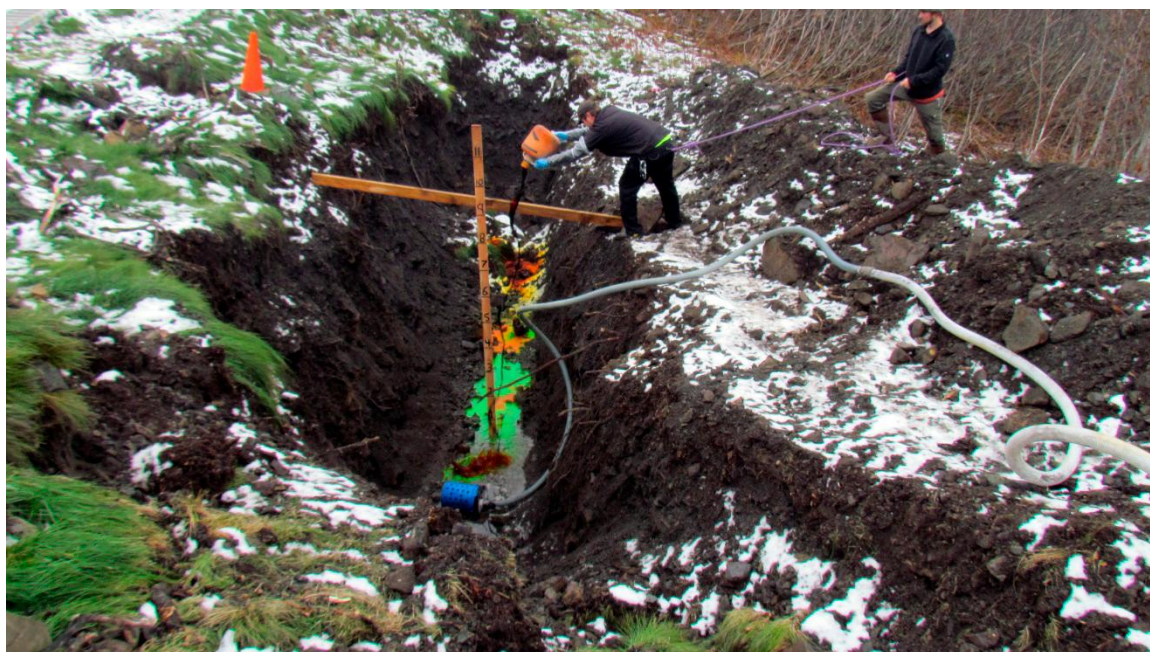
Figure 24 - Fluorescein introduction into a trench in alluvium, showing safety rope, staff gauge, hose leading from a meter measuring flow rate, and blue diffuser in bottom of trench. The diffuser is designed to minimize erosion of the sides of the trench (thus reducing sediment in the infiltrating water). The trench bottom is level and 9.1 m (30 ft) long, 1.1 m (45 in) wide, and 3.4 m (11 ft) deep on the uphill side. The trench accepted 18,900 liters (5,000 gal) of water and fluorescein dye at a mean rate of 92 L (25 gal) per minute.
